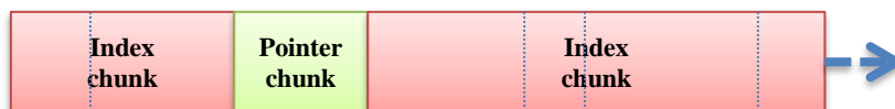
Figure 2: Structure of the chunk based archive generated for a function call similar to that shown in Listing 2, dotted lines delimit how individual sub-elements might be aligned within the index chunks. Pointer chunks always contain a single {pointer, size} entry.
