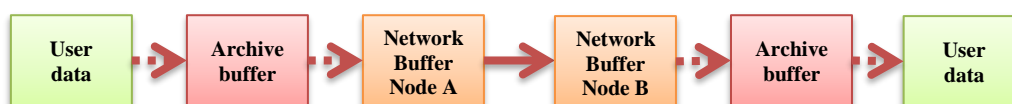
Figure 1: Memory copies that can occur when transferring data from user variables on one node to another.
